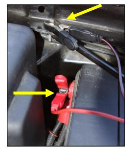
Connect red clip to 12V-DC power. Connect black clip to chassis ground.
