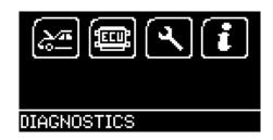
Connect the SD-MAT Tool to a vehicle using the 16 Pin Diagnostic plug. The SD-MAT Tool will then power up and take you to the Main Menu screen.
