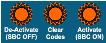
1. If there is an error in communications with the SBC system then all three lights will flash.
